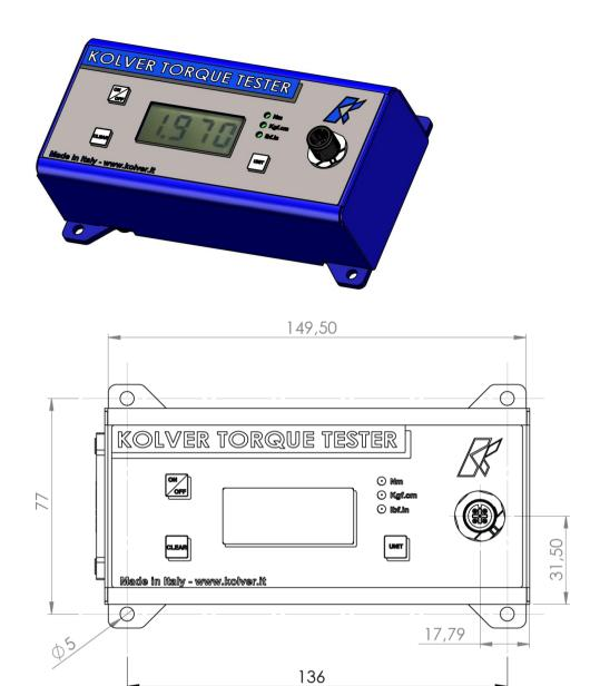
Example of MINI KE + KT series external cell + joint simulator
